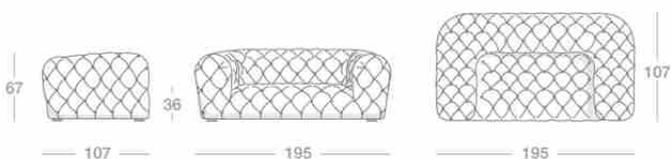
Quilted button back model. Structure in fir plywood. Seat frame in fir. Base in wenghé-stained beech. Differentiated density polyurethane foam filling with acrylic fibre covers. Springing with woven elastic straps of covered rubber.
