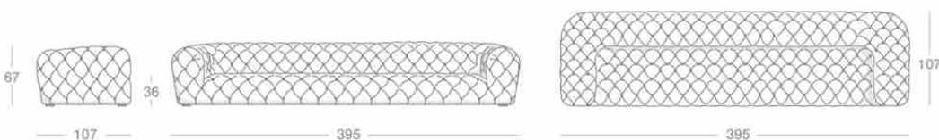
Quilted button back model. Structure in fir plywood. Seat frame in fir. Base in wenghé-stained beech. Differentiated density polyurethane foam filling with acrylic fibre covers. Springing with woven elastic straps of covered rubber.
