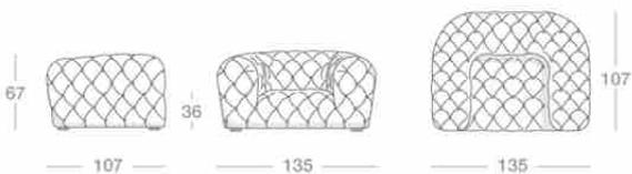
Quilted button back model. Structure in fir plywood. Seat frame in fir. Base in wenghé-stained beech. Differentiated density polyurethane foam filling with acrylic fibre covers. Springing with woven elastic straps of covered rubber.
