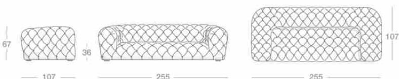
Quilted button back model. Structure in fir plywood. Seat frame in fir. Base in wenghé-stained beech. Differentiated density polyurethane foam filling with acrylic fibre covers. Springing with woven elastic straps of covered rubber.
