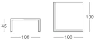
Frame in unfinished tubular metal and top in 25/10 black sheet metal. Visible weld and smoothing, **with antirust protection with clear matte enamel and wax finish or, on request, finish with oxidizing material and protection with varnish for a soft effect.**
