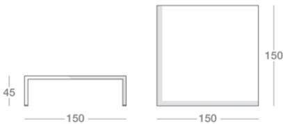
Frame in unfinished tubular metal and top in 25/10 black sheet metal. Visible weld and smoothing, **with antirust protection with clear matte enamel and wax finish or, on request, finish with oxidizing material and protection with varnish for a soft effect.**
