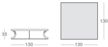
**Frame in hand-finish burnished or, on request, natural satin-finish with matte varnish steel.** Double base consisting of 10 mm thick, laser cut arches, welded onto structural cross rods. Top in 20 mm thick marble with wood underside.
